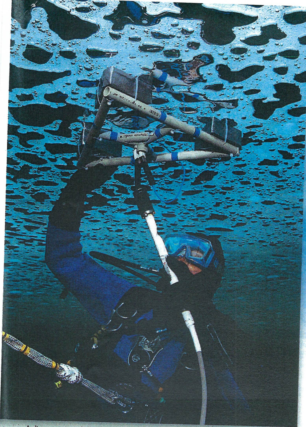
A diver measures light penetration through sea ice in the Arctic Ocean.
